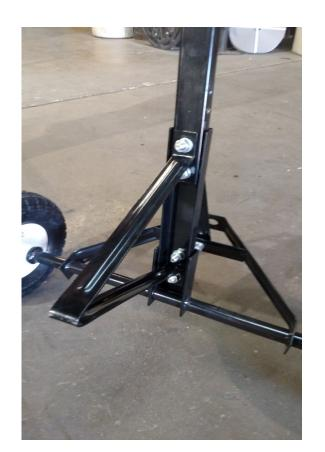
Next, mount the tank support onto the handle with the ½" head 2 ½" long
