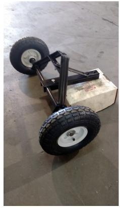
Next assemble the handle to the main frame using the longer 11/16" bolts. Ensure that the support leg is attached to the front-most bolt and the rear-most bolt.
