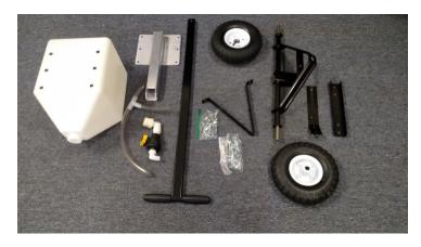
Then begin assembly of the buggy by adding the braces and wheels to the main framework. Leave the shorter 11/16" head bolts and larger ¾" bolt very loose at this point. Use cotter flat washers and cotter pins to secure wheels on axles.
