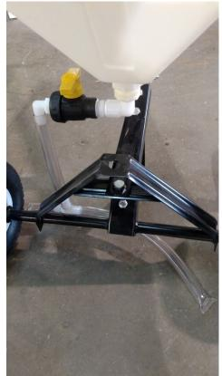
Then start at the short end of the boom using the enclosed zip ties to attach the boom to the under side of the axle. NOTE- The tube boom can be rotated To facilitate installation. Use care to not block any of the dispersing holes, and assure holes are facing downward.
