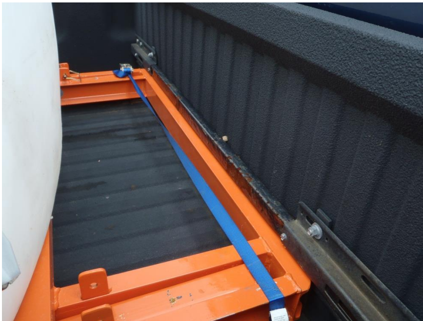
If you have to drive long distances with the tank unloaded put a small ratchet strap (blue in the pic) across the front of the frame to keep it from bouncing or shifting.
