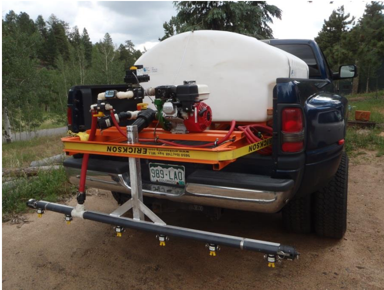
Pic 4- Boom in “use” position. Boom’s vertical brace should clear the bumper by at least 3/4”
