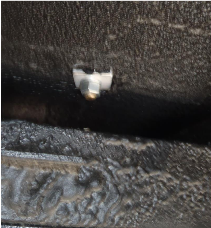
Pic 6 A 1.5 inch square of strap steel acting as a washer under the bed for a main mounting bolt.
